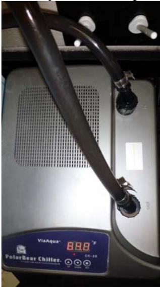
The vinyl hose from the water pump outtake is then connected to the chiller intake port. The vinyl tubing pushes down onto the port inlets, lubricating the inlet barb helps (use warm water). Push the tubing all the way onto the port and make sure it is well seated.
